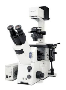
Inverted optical microscope with dark field condenser. Equipped with halogen and mercury lamps for fluorescence spectroscopy.
