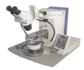
This instrument is a multipurpose semiautomatic wire bond tool for R&D purposes.
