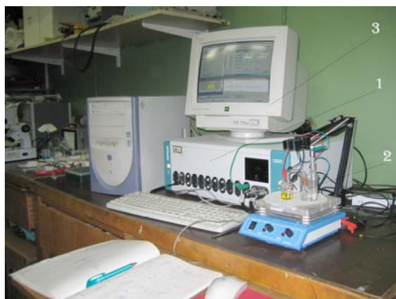
1 – Autolab PGSTAT30, 2 – electrochemical cells, 3 – computer.
