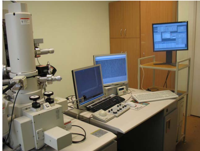
FE SEM Hitachi S4800/Raith EBL system ELPHY Quantum Version 4.0
